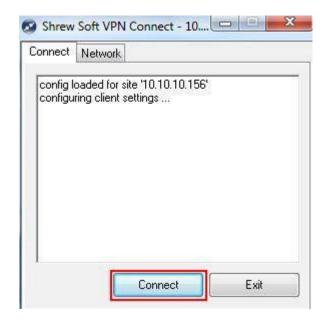
Step 12: After Shrew Soft VPN show tunnel enabled as the followings, you need ping TL-ER6120 LAN IP.
