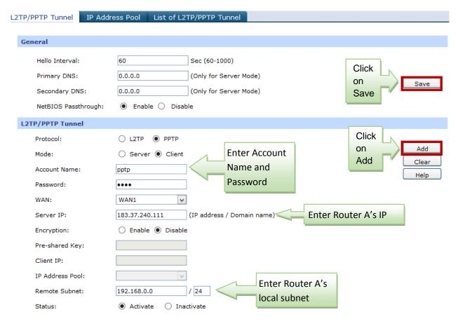
Step 3: Under Server IP, enter Router A's IP address, which is 183.37.240.111.
