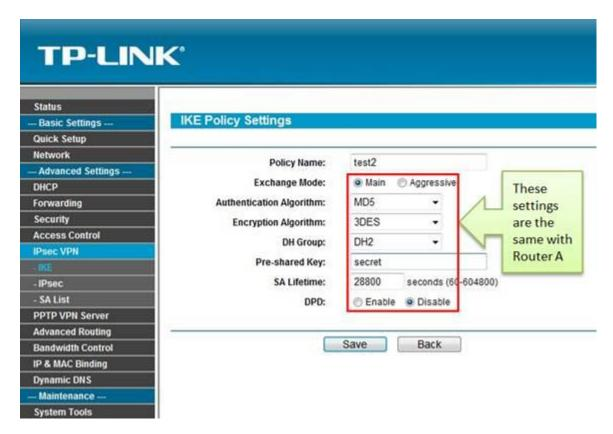
Step 3: Authentication Algorithm and Encryption Algorithm are the same with Router A, we use MD5 and 3DES in this example.
