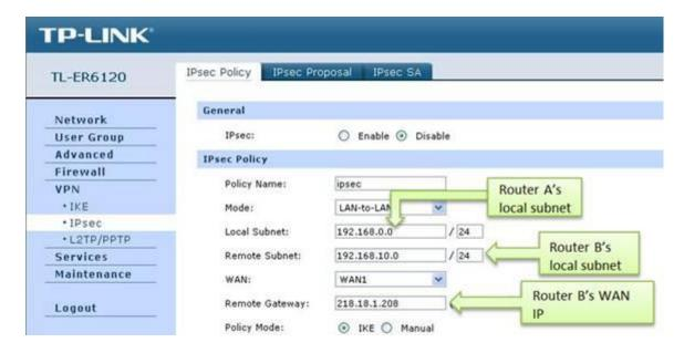
Step 9 : Select WAN you use and type in Remote Gateway. In this example, the Remote Gateway is Router B's WAN IP address, 218.18.1.208.
